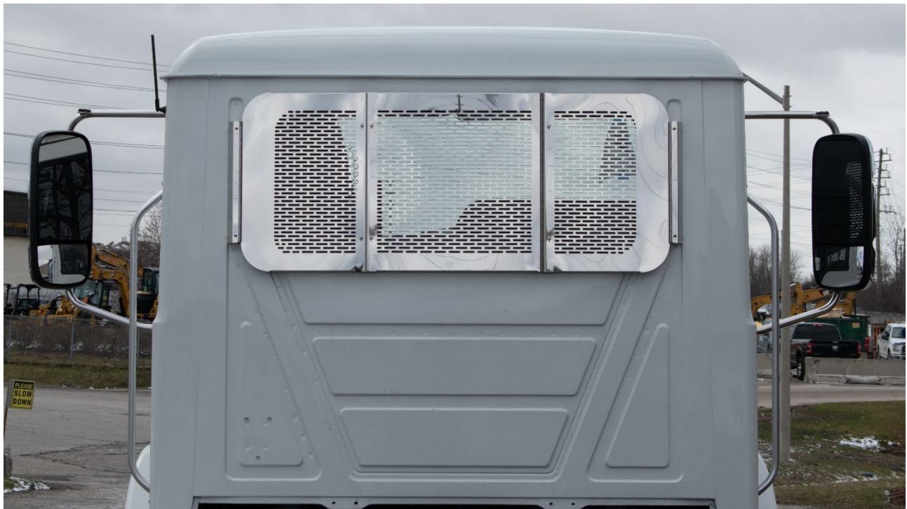
Figure 11: Finished Rear Window Guard Installed
