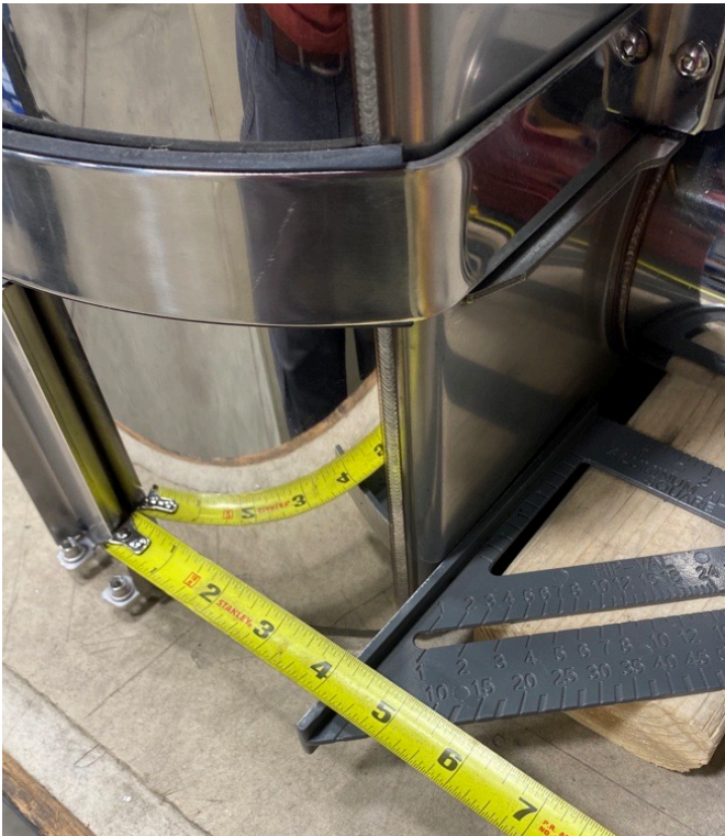
Figure 7: Measuring Rear Bracket Position (Driver Side)
