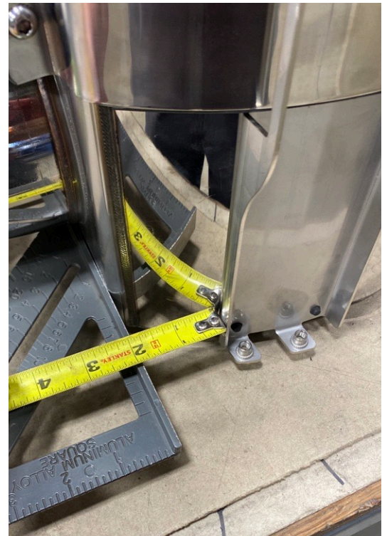
Figure 8: Measuring Front Bracket Position (Driver Side)
