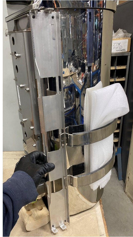
Figure 5: Front Bracket Orientation (Driver Side Shown)
