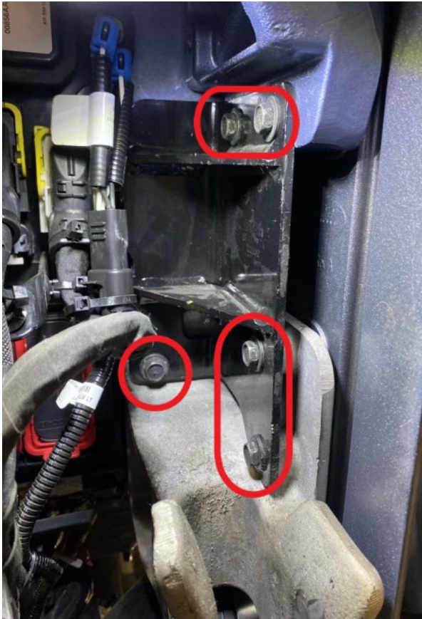
Figure 2: First 5 Bolts to Remove (Driver Side Shown)
