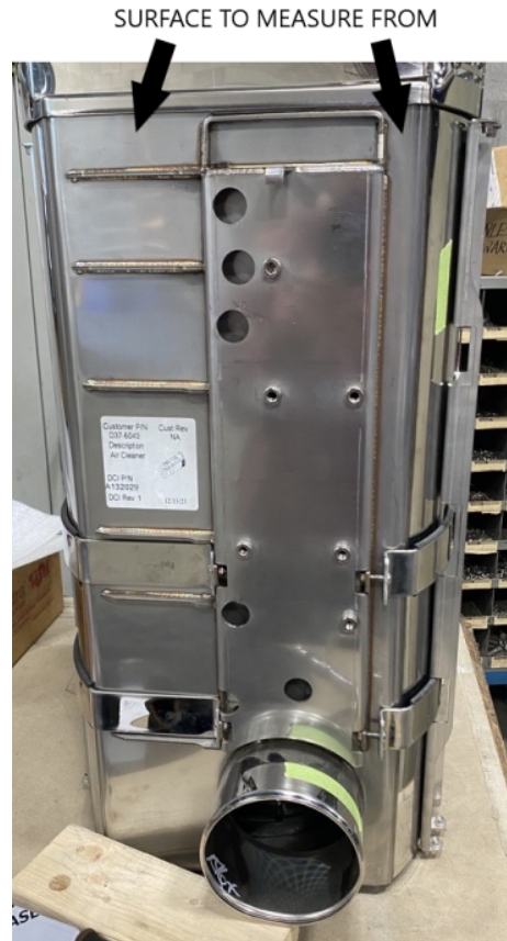
Figure 6: Surface to Measure from when Positioning Brackets (Driver Air Cleaner Shown)
